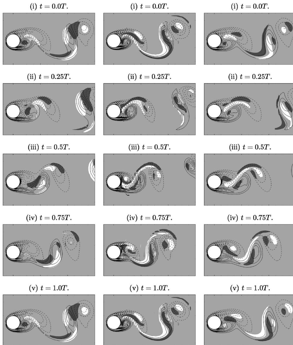
FIG. 2. A comparison between the perturbation fields obtained during one shedding cycle for each of the modes A, B, and C instabilities [(a), (b), and (c), respectively]. Arbitrary contour lines show the base flow vorticity (dashed lines denote negative vorticity), and positive and negative spanwise vorticity in the perturbation field is shaded white and black, respectively.
