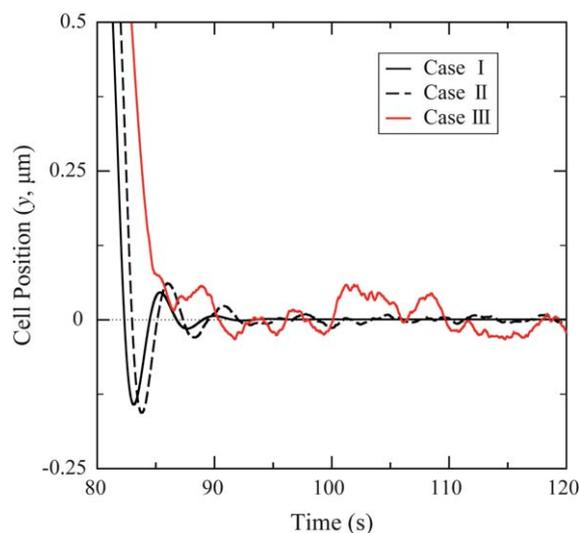
**Fig. 3** Controlling the position of the cell using fluid flow. By adjusting the relative flow rates in the device, and therefore moving the saddle point, the flow velocity can be used to direct the cell. Based on this principle, a feedback control system can be used to position the cell and stabilise the system. Response curves show the  $y$  (vertical) position of the cell vs. time for case I (solid line); case II (dashed line) and case III (grey line).
