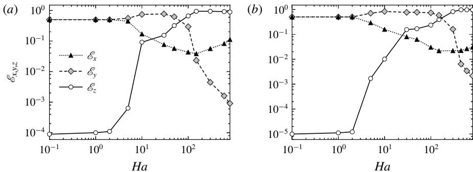
FIGURE 7. Distribution of initial eigenvector energy across horizontal  $\mathcal{E}_x$ , vertical  $\mathcal{E}_y$  and streamwise  $\mathcal{E}_z$  velocity components (i.e.  $u, v$  and  $w$ ), as a function of  $Ha$  for (a)  $Re = 5000$  and (b)  $Re = 15000$ . Energy magnitudes are normalised using the total perturbation kinetic energy.
