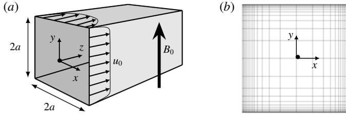
FIGURE 1. (a) Flow configuration for the straight duct with square cross-section and (b) an example graded spectral element distribution in the  $x$ - $y$  plane for three-dimensional investigations at  $Ha = 30$ . The Shercliff and Hartmann boundary layers respectively develop on the vertical and horizontal side walls.
