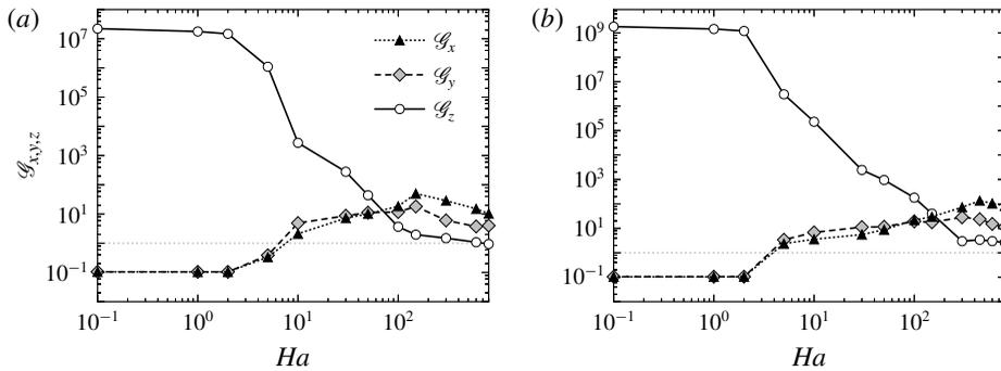
FIGURE 9. Amplification of perturbation kinetic energy  $\mathcal{G}_x$ ,  $\mathcal{G}_y$  and  $\mathcal{G}_z$  in the horizontal, vertical and streamwise velocity components (i.e.  $u$ ,  $v$  and  $w$ ), respectively, as a function of  $Ha$  for (a)  $Re = 5000$  and (b)  $Re = 15000$ .
