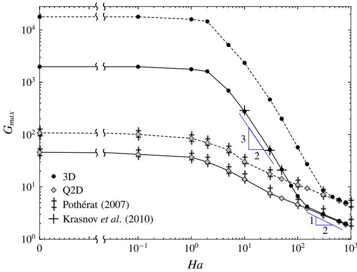
FIGURE 2. (Colour online) Optimal transient growth as a function of Hartmann number for both three-dimensional and quasi-two-dimensional models at  $Re = 5000$  (—) and  $15000$  (---). Also provided are the optimal transient growths predicted by Krasnov *et al.* (2010) using a three-dimensional analysis, and by Pothérat (2007) using the SM82 model. The horizontal axis is logarithmically and linearly scaled for  $Ha \geq 2.2 \times 10^{-2}$  and  $Ha < 2.2 \times 10^{-2}$ , respectively.
