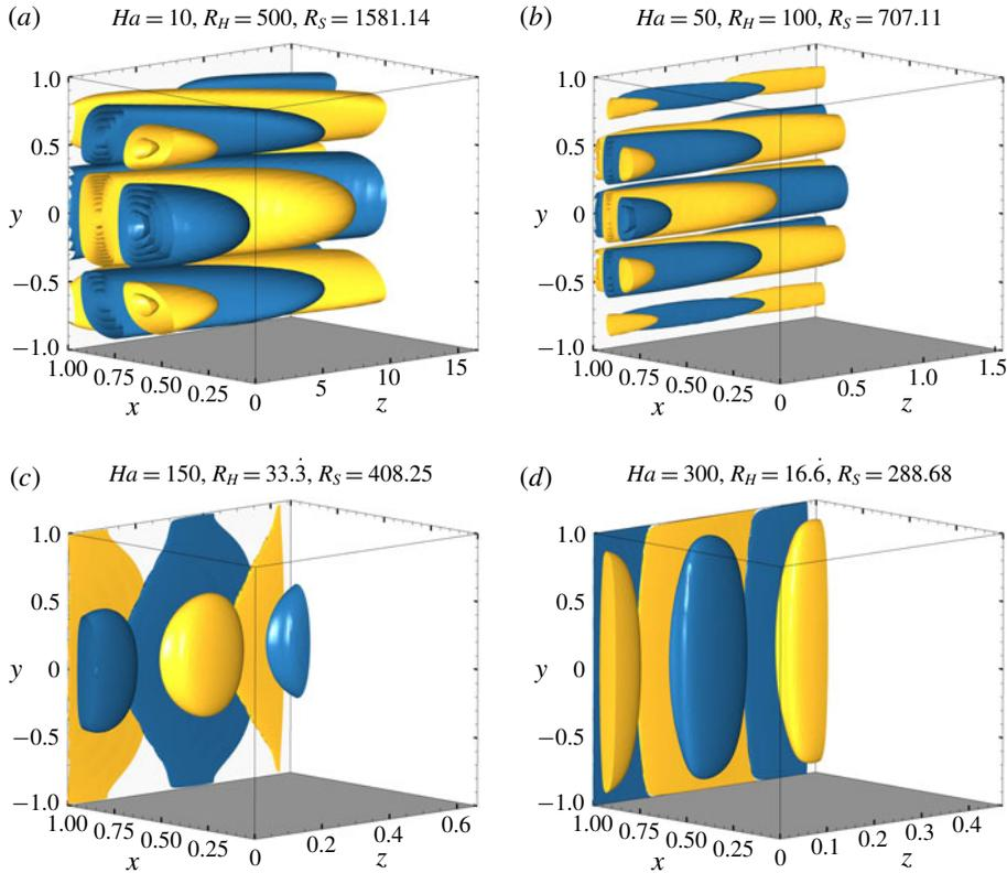
FIGURE 10. (Colour online) Vertical component of vorticity  $\omega_y$  iso-surfaces of the perturbation fields at time of maximum transient amplification  $\tau_{opt}$  for (a–d)  $Ha = 10, 50, 150$  and  $300$  at  $Re = 5000$ . Iso-surfaces specified as per figure 5.
