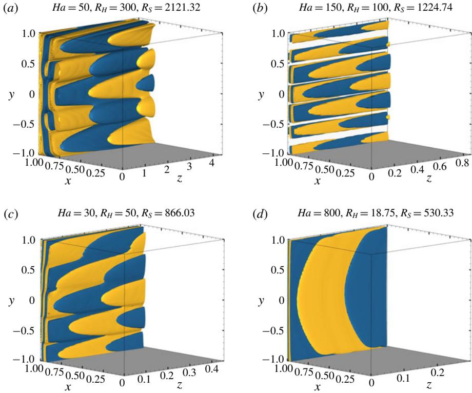
FIGURE 6. (Colour online) Vertical component of vorticity  $\omega_y$ , iso-surfaces of the optimal eigenvector fields producing maximum transient amplification  $G_{max}$  for (a–d)  $Ha = 50, 150, 300$  and  $800$  at  $Re = 15000$ . Iso-surfaces specified as per figure 5.
