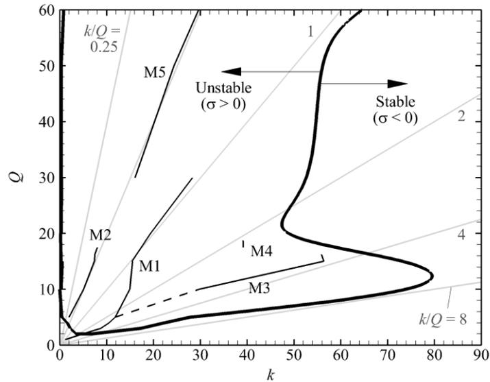
**Figure 1.** Neutral stability (solid line) and loci of maximum growth rate (dashed lines) for the five identified mode branches (labelled) across the  $Q$ – $k$  parameter space for  $Ra = 10^9$  and  $Pr = 6.14$ . For guidance, the data is plotted over faint radial lines of constant  $k/Q$ , with values doubling in the clockwise direction from  $k/Q = 0.25$  to 8.
