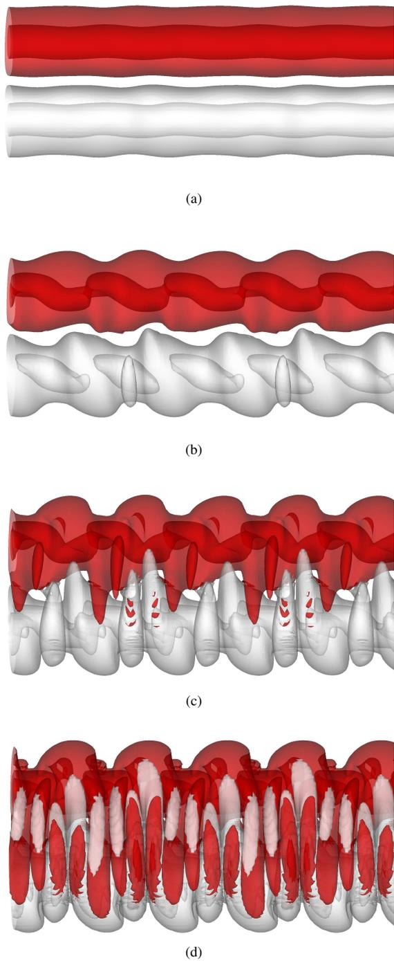
Figure 3: Snapshots showing isosurface contours of vorticity during the development of mode [-1,1]. The lower vorticity contours ( $|\omega| = 0.5$ ) have been rendered semitransparent to reveal the upper vorticity contours ( $|\omega| = 3.0$ ). Negative vorticity isosurfaces are shown in red, positive vorticity isosurfaces are shown in white. Snapshots correspond to: (a),  $t^* = 16.65$ ; (b)  $t^* = 20.25$ ; (c),  $t^* = 22.05$ ; and (d),  $t^* = 23.4$ .
