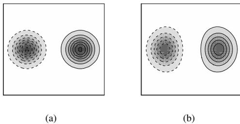
Figure 2: Vorticity contours,  $\omega_z$ , showing the evolution of the initial flow field to the final, 'relaxed', elliptical profile of each vortex core used for later three-dimensional simulations. Figure (a) shows the initial field comprising two vortices of Gaussian profile. Figure (b) shows the flow field at the completion of the relaxation process.
