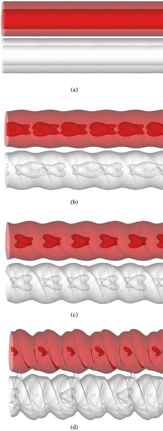
Figure 5: Snapshots showing isosurface contours of vorticity during the development of mode  $[-2,0]$ . The lower vorticity contours ( $|\omega| = 0.5$ ) have been rendered semitransparent to reveal the upper vorticity contours ( $|\omega| = 2.5$ ). Negative vorticity isosurfaces are shown in red, positive vorticity isosurfaces are shown in white. Snapshots correspond to: (a),  $t^* = 20.25$ ; (b)  $t^* = 31.5$ ; (c),  $t^* = 33.75$ ; and (d),  $t^* = 40.5$ .
