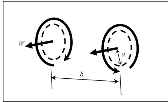
Figure 1: Schematic representation of the flow field under investigation. Here,  $a$  is the characteristic core radius,  $b$  is the separation distance between the vortex cores and  $W$  is the velocity component parallel to the axial direction.
