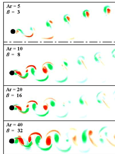
Figure 4. Streamwise vorticity of the perturbation field for the dominant mode associated with a “Mode A” spanwise wavelength for each ring. All simulations at  $Re = 250$ . Red indicates positive vorticity, and green is negative vorticity. Dashed line represents axis, ring cross-section represented by black circle, and flow is from left to right.
