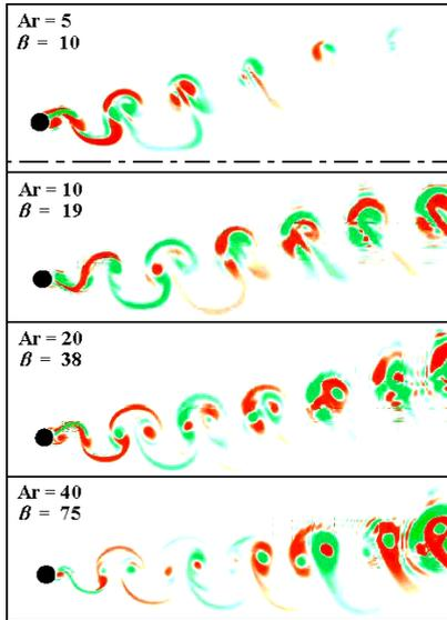
Figure 5. Streamwise vorticity of the perturbation field for the dominant mode associated with a “Mode C” spanwise wavelength for each ring.  $Ar = 5$  at top to  $Ar = 40$  at bottom.  $Ar = 5$ ,  $Ar = 10$  at  $Re = 250$ ,  $Ar = 20$  and  $Ar = 40$  at  $Re = 400$ . Vorticity contours are between  $-0.5$  and  $0.5$ . Axis indicated as dashed line if shown.
