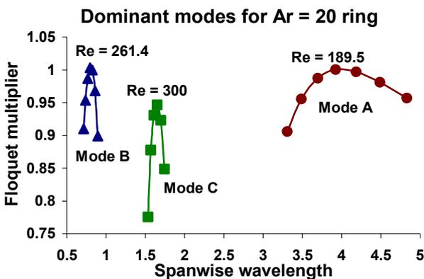
Figure 3. Floquet multiplier profiles for the  $Ar = 20$  ring. Note the Reynolds numbers for each local maximum, and the spanwise wavelength at which it occurs.
