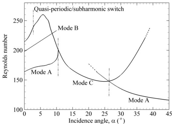
Fig. 5 The updated regime map for linear instability modes in the wakes behind inclined square cylinders, with critical Reynolds number curves plotted against incidence angle. The various modes are labelled, and dash-dotted lines are used to mark important incidence angles in the parameter space. The terms "QP" and "C" refer to the quasi-periodic and subharmonic (Mode C) parts of that transition curve.
