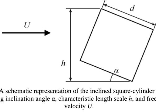
Fig. 1 A schematic representation of the inclined square-cylinder system, showing inclination angle  $\alpha$ , characteristic length scale  $h$ , and free-stream velocity  $U$ .
