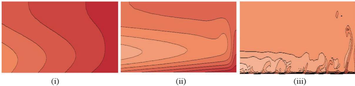
**Figure 2.** Temperature contours focused on the hot-end of the enclosure for  $A=0.04$  (i) diffusive  $Ra=10^8$ , (ii) transition  $Ra=10^{10}$  and (iii) convective  $Ra=10^{12}$  regimes. The darker colour sheds refer to higher temperatures.
