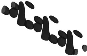
As the base vortex pair is brought still closer together (Fig. 9(c)), we see an increase in the relative strength of the central coupled region compared to the maximum perturbation vorticity in the vortex plane. This is shown in the progression of contours in Figure 9(a)–(c). The relative increase in the strength of the central coupled region with respect to the vortex core region amplifies the coupling effect.
