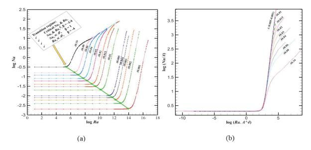
Figure 1. Plots of (a) log Nu against log Ra and (b) log (Nu/A) against log ( $RaA^4$ ), for various aspect ratios between A=0.001 to 0.16.
