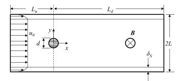
FIG. 1. Schematic diagram of the numerical domain. The shaded area indicates a cylinder of infinite extension along the out-of-plane z-axis with diameter d.
