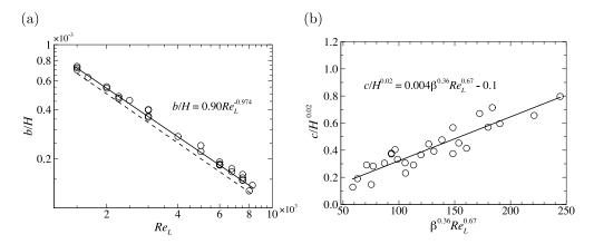
FIG. 7. (a) A plot of b/H against  $Re_L$  and (b)  $c/H^{0.02}$  against  $\beta^{0.36}Re_L^{0.67}$  measurements (symbols). The solid lines in (a) and (b) are a power-law fit and a linear fit, respectively, to the data adopting the equations shown, and the dashed line is the behaviour described by the Hartmann friction term  $(H/Re_L)$  for comparison.
