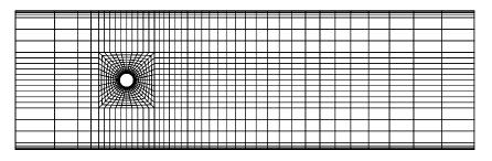
FIG. 4. Macro-element distribution. Fine resolution was placed at the proximity of cylinder surface and walls to ensure accurate representation of the thin boundary layers and the expected wake structures.
